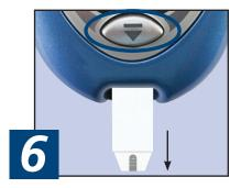
Hold Meter with Test Strip pointing down. Press Strip Release Button to discard Test Strip in the appropriate container.
